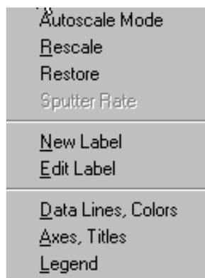
The “Graph” menu controls the data display functions. Data scales can be customized for comparison to previously recorded data. Labels on the charts and how the data is displayed can also be customized so that all data is displayed with the same scale expansions.
