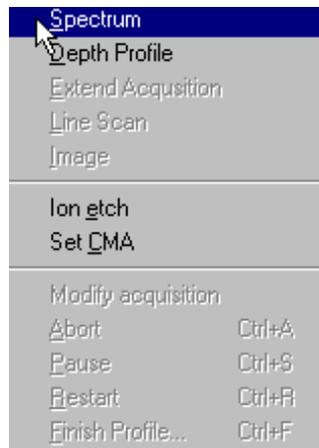
Other controls let you abort an acquisition, pause it, or simply restart from the lowest energy. Depth profiles can be extended or terminated after the current data collection scan and line scans and images (for multiple elements with background subtract) can be initiated.
