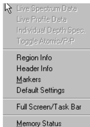
The “View” menu lets the operator restore live data as well as display information about the data collection process. For comparison purposes, existing data in the data collection computer or data on the local area network can be displayed against the data being accumulated. When depth profiling the ion sputter rate can be changed for different materials within the sample.
